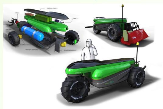
First proof of concept: manual operation with a radio joy stick and completely electrically driven from a 30 kWh battery pack
