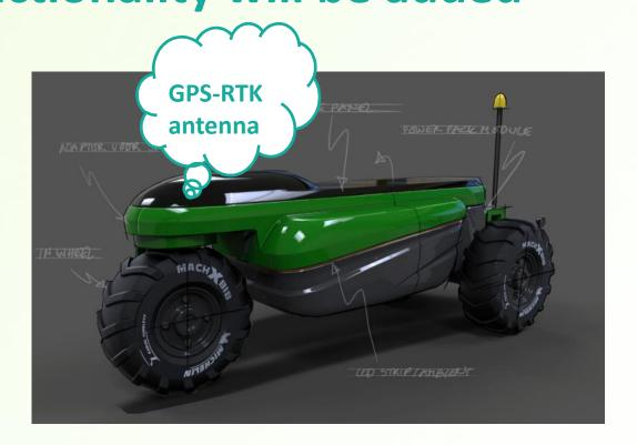
The eTrac-20 is prepared for GPS-RTK for unmanned navigation with an accuracy of 2 centimeters for precision farming applications.
