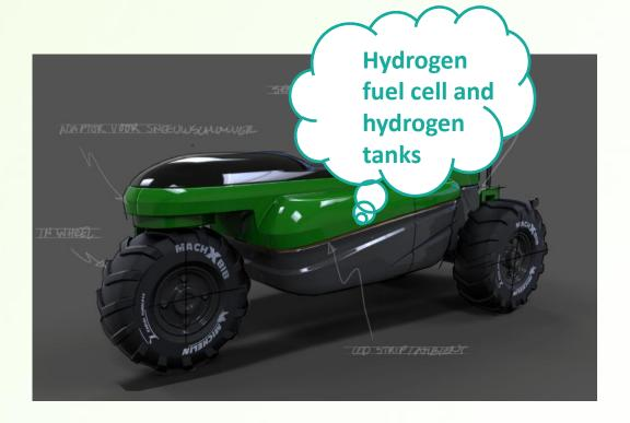
The eTrac-20 is prepared to run on hydrogen. A hydrogen fuel cell and hydrogen tanks will be added with prototype #2 for range extension.
